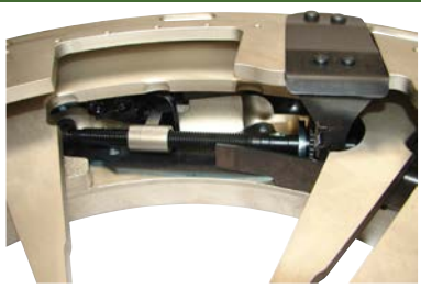
The adjustment mechanism of the LuK travel-adjusted clutch.
