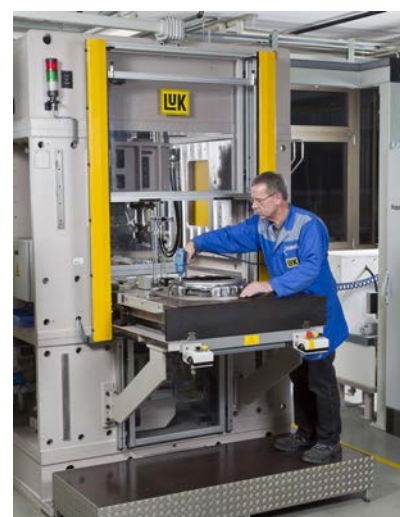
Fixation of the clutch on the test measurement stand (relative load, clamp load, load curve and lift).
