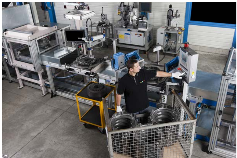
LuK Truckparts – Commercial Vehicle Competence Center – with full vertical manufacturing integration. This picture depicts the new production line for the LuK Travel Adjusted Clutch (TAC) 395 mm (push-type) used in the Mercedes-Benz Antos.
