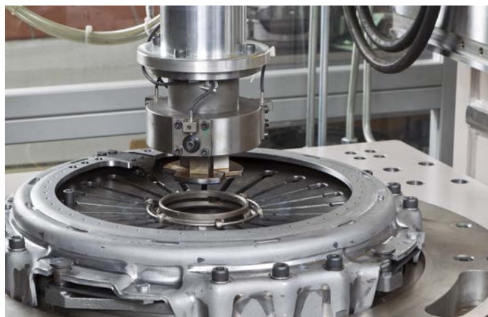
The clutch is fast engaged repeatedly to test its load capacity
