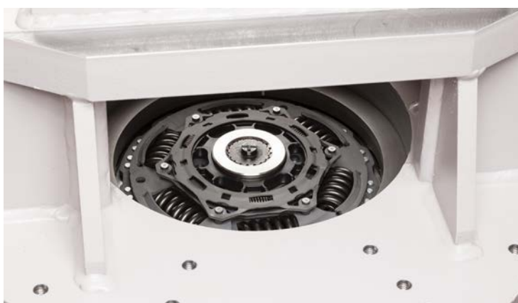
The clutch disc of the LuK Travel Adjusted Clutch (TAC) – here torsion damper performance is being measured.
