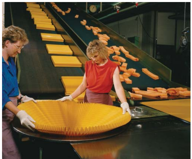
The star-shaped pleat of the paper filter elements enabled maximum filtration performance in even the smallest of spaces
