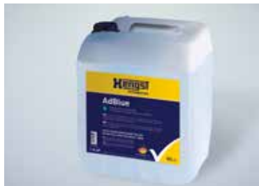
DEF needs to be kept clear of all contaminants. Steel drum reacts with the solution resulting in rust impurities. Cool and ventilated storage is required for optimal shelf life
