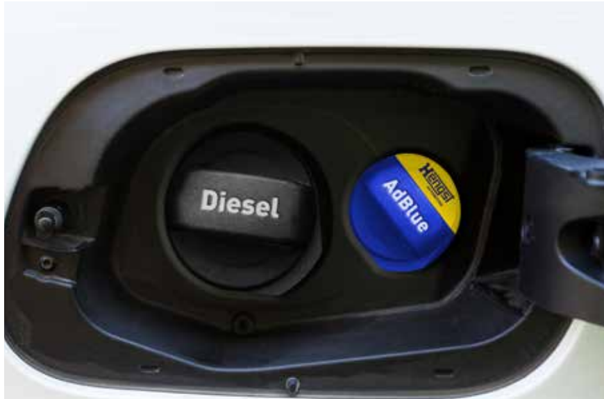
Using an approved DEF is as important to the engine as using a proper diesel for the engine. Non approved DEF might result in not meeting required emission level
