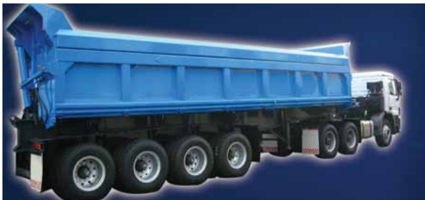
Typical 7-axle side tipping trailer-tractor combination with Knorr-Bremse conventional trailer brake kit for the mining application in Kalimantan, Indonesia
