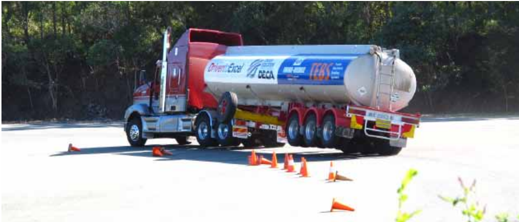
Tractor and trailer without RSP function when making a sharp unplanned turn
