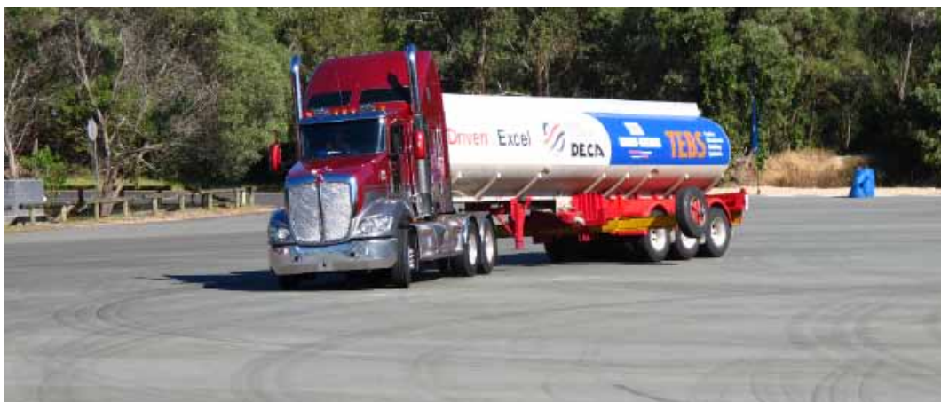
Tractor and trailer equipped with TEBS and RSP function when making a sharp unplanned turn
