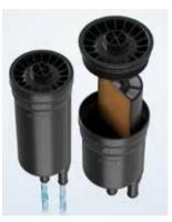
Smart filtration technologies can also protect the core components of the fuel cell from gases and particles. Hengst has designed a cathode filter for this purpose, which separates sulfuric gases and ammonia in a particularly effective manner, thereby preventing damage to the catalyst and the fuel cell membrane.
